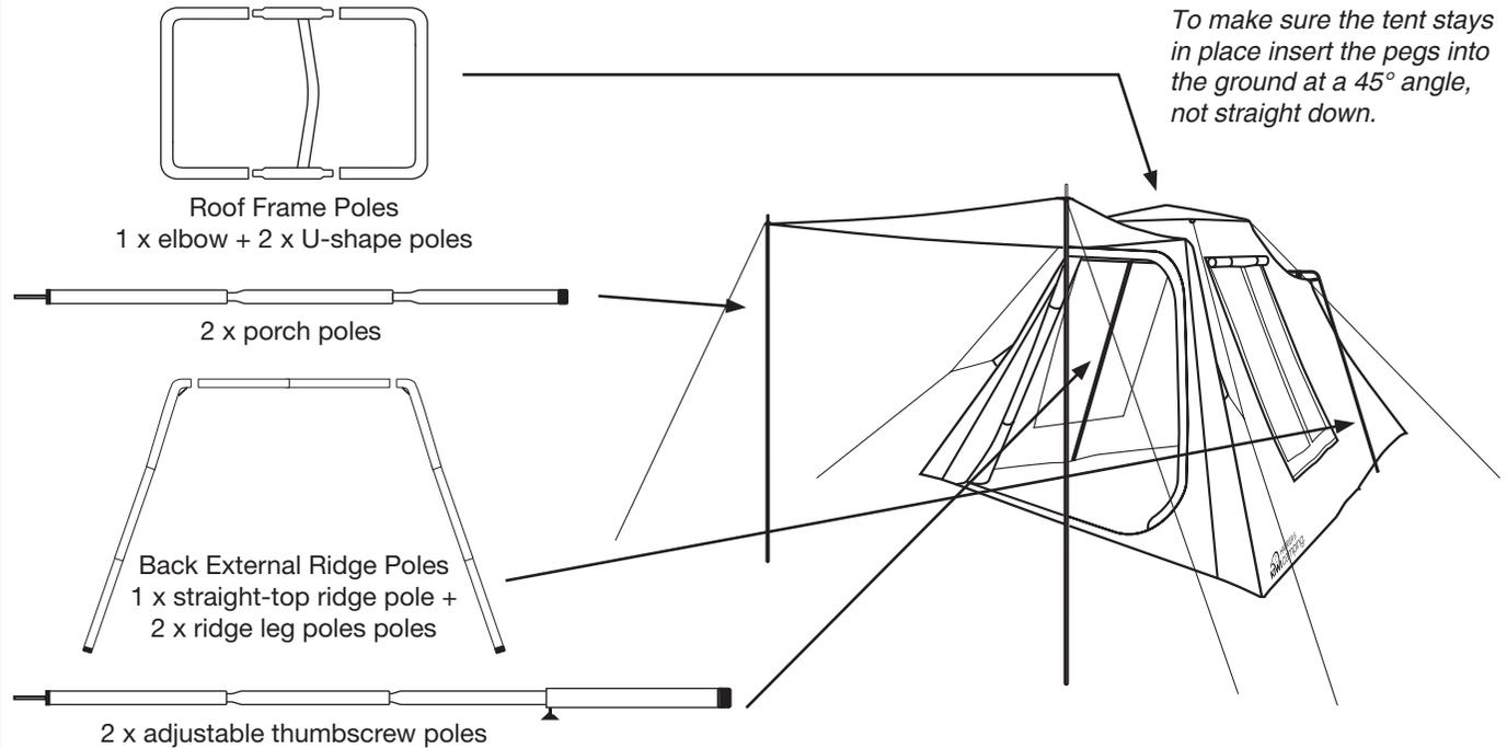
1. Select a dry, level site and clear any sharp objects that may puncture the floor. Remove the tent from its carry bag, untie fabric ties and unroll the tent.
