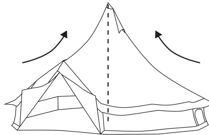
4. Inside the tent assemble the remaining poles into an A frame for easier installation. Insert the top pin on the A frame and bend through the eyelet at the top of the door opening.
