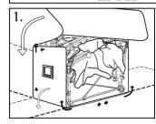
Unzip storage case completely before inflation, make sure panel of storage case is laid flat on the floor, this will prevent damage to bed frame and ensure smooth extension out of its storage case.
