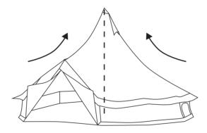
5. Inside the tent assemble the remaining poles into an A-frame for easier installation. It is easier to install the A-frame if the poles are not fully extended. Insert the top pin of the A-frame through the eyelet at the top of the door opening. Place the pole-tip hat on top of the pole on the outside of the tent to stop any water seeping in.
