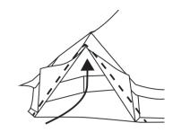
7. Peg out all the guy ropes and tighten with tri-tensioners to ensure they are taut.
